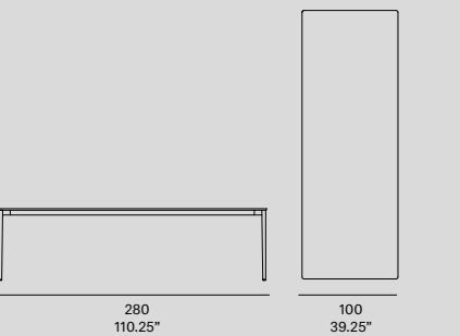
**[en]** Structure made of stainless steel tube, finished with polyester powder. The collection is available in European oak veneer top and lacquered top version (MDF). Tabletop thickness: 19 mm/0.75" thick for expandable and round dining tables, 12 mm/0.47" thick for square dining tables. Delivered unassembled.
