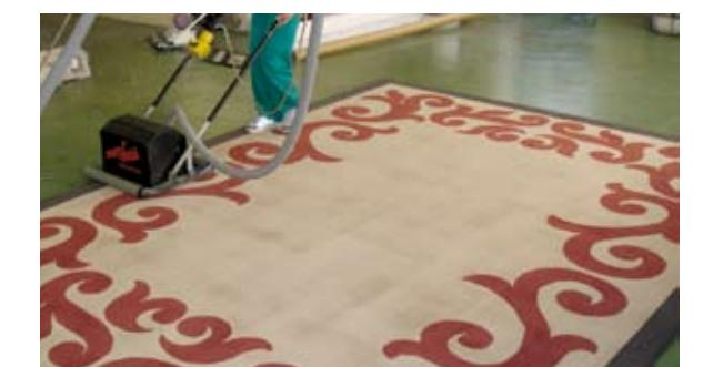
**18. Tundido** | Shearing | Rasage
