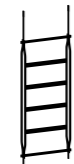
cod. 16.68 cm L 90 x P 34 x H 240 min cm L 90 x P 34 x H 330 max inch L 35.4 x W 13.4 x H 94.5 min inch L 35.4 x W 13.4 x H 129.9 max
